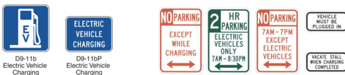
Figure 5.3: Sample Signs Recommended by US Federal Highway Administration
